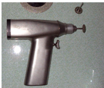
Figure 2. A 30 mm diameter diamond tipped cutting disk mounted in a Stryker drill.
