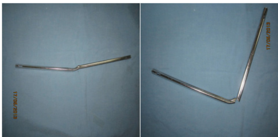
Figure 4. The bent intramedullary nail cut and removed intact, showing a remaining bridge of metal.
